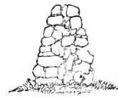
Fig. 6.—Cross Section of a badly built wall.
